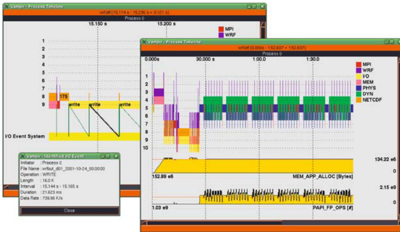
Fig. 5 Complete Process Timeline of a WRF process (right). By means of the call stack representation, one can clearly see the initialization phase and the iteration steps. It includes performance counters for memory allocation and floating point operations per second. A zoomed version shows individual I/O operations with very slow speed indicating a performance problem (left)
